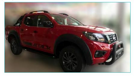
PESOS Vehicle weight, kg 2,034 Gross vehicle weight, kg 2,910 TIRES Tires 255/60 R18 **DIRECTION SYSTEM** Type of address Hydraulic assistance **SUSPENSION** Lead Double fork Rear 5-arm with rigid axle and stabilizer bar BRAKES Forwards Ventilated disc Rear Drum **ELECTRIC SYSTEM** Alternator (Amps) 120A Ignition type Electric
